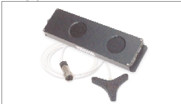
Miniaturized scanner unit containing system electronics with head-mountable sensor (foreground).
