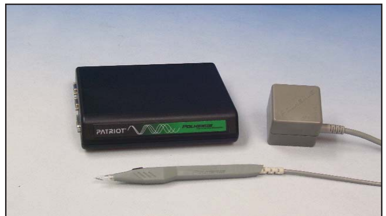
Standard PATRIOT Digitizer includes TX2 Source, 8" stylus (shown above) and foot/hand switch (as seen on the back page)
