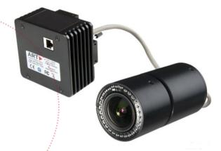
ART's unique new camera specially adapted for outdoor applications such as in-car tracking systems. It consists of 10nm narrow bandpass interference filter. Narrow bandpass interference filter makes possibility of tracking even in daylight.
